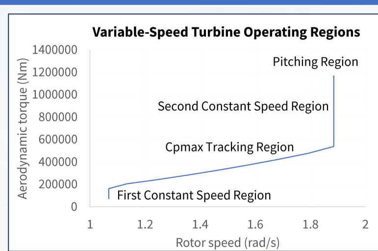
Keep the turbine work at its optimum condition. Four different regions of the graph:
