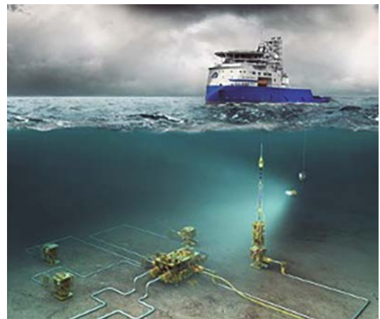
Lett brønnintervensjon – RLWI © Leverandør FMC Technologies https://ndla.no/image/26? CC BY-SA 4.0 DEED "Light well intervention – RLWI"
