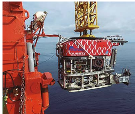
The submersible vehicle MARUM-QUEST is lowered into the water from the stern of the RV METEOR © MARUM - Zentrum für Marine Umweltwissenschaften, Universität Bremen; V. Diekamp ( https://www.marum.de/Entdecken/Technologien.html ). CC-BY-4.0
