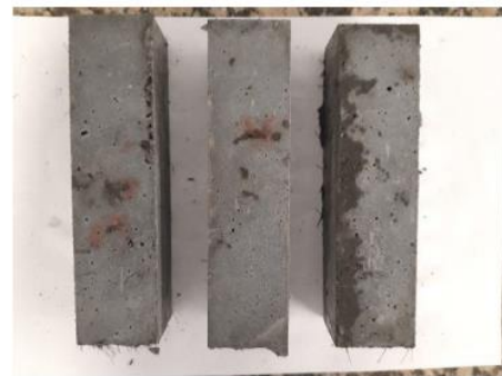
Appearance of concrete samples with microfibres
