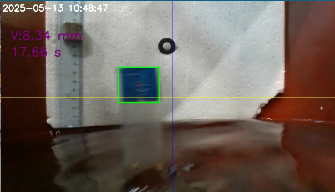
Sloshing becomes dominant with no porous mesh specially at the first second due to sudden acceleration.
