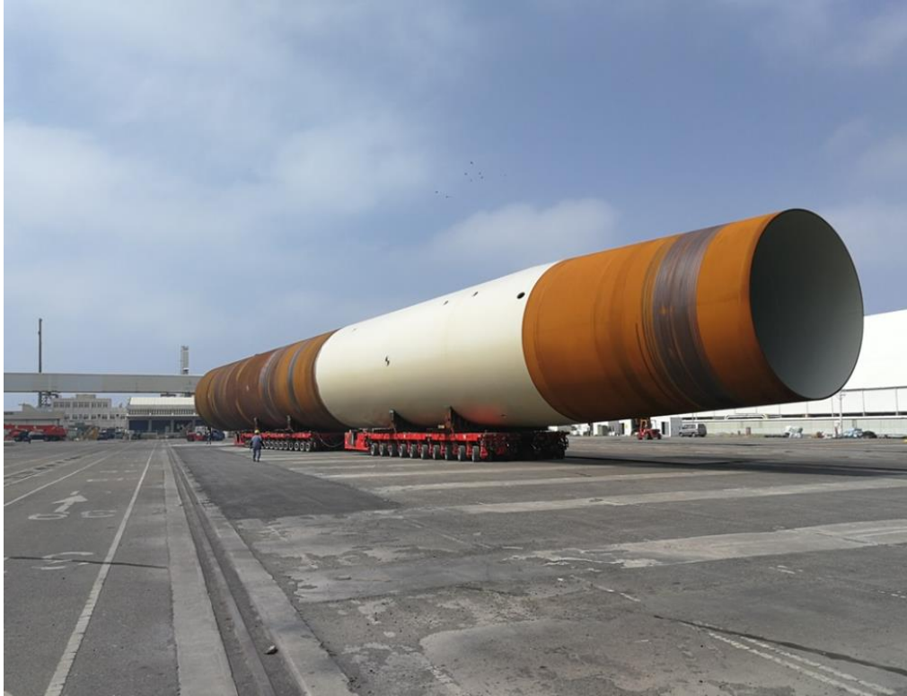
beyond XXL" monopile for the Yunlin offshore wind farm (image: Steelwind Nordenham, FHI corporation, via offshorewind.biz)
